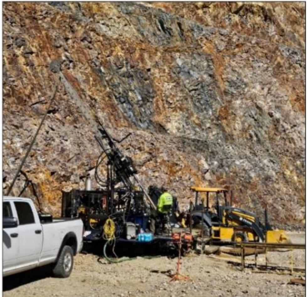
Figure 1 Company owned diamond core drill rig mobilised to the Colosseum and drilling inside the Colosseum South pit.
