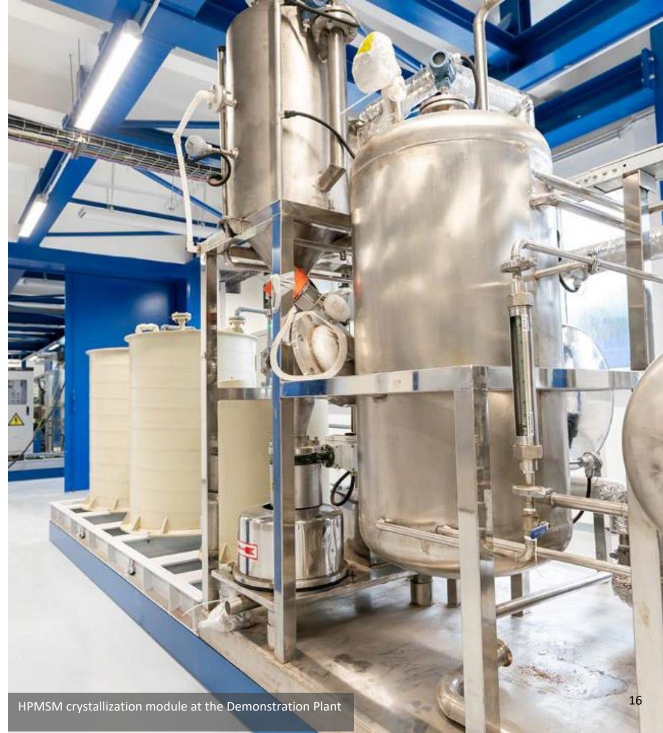
HPMSM crystallization module at the Demonstration Plant
