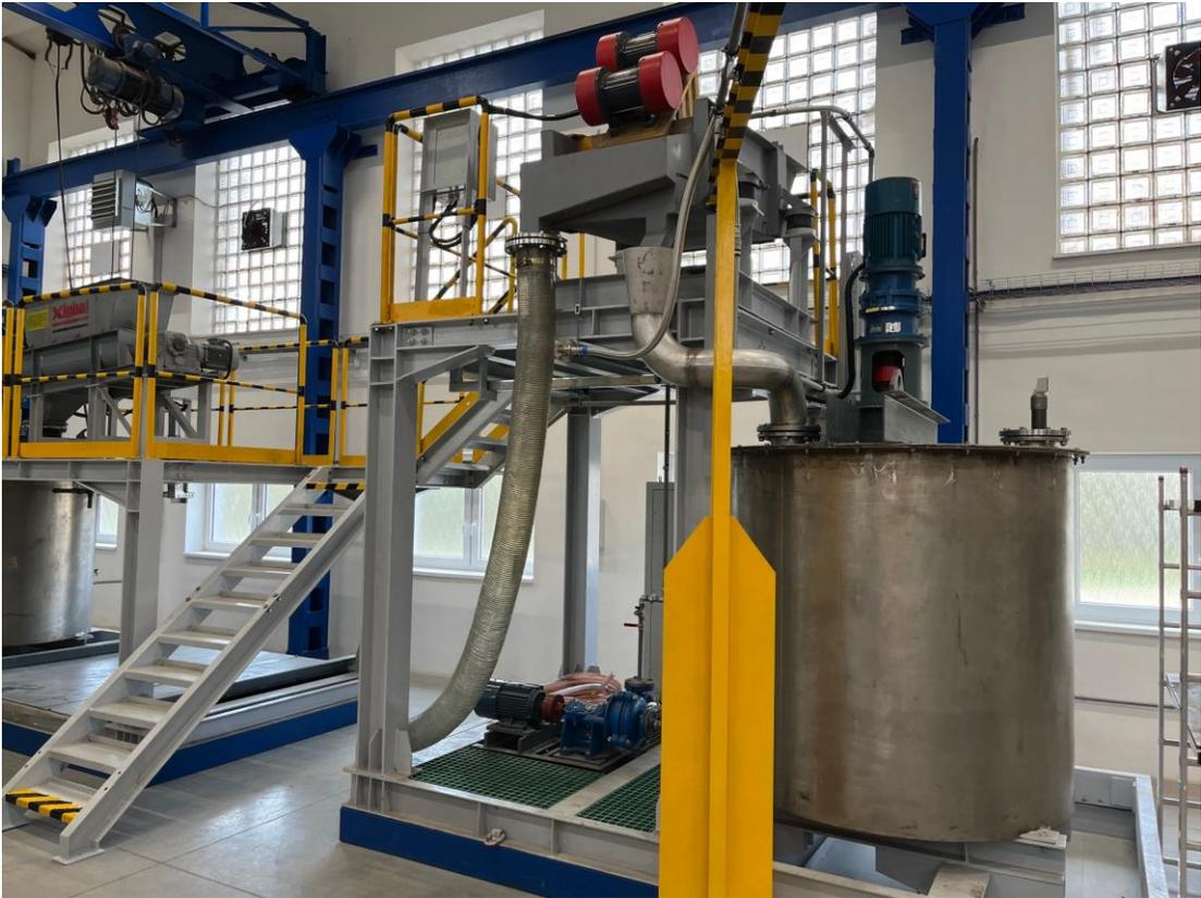
**Photo 1. Ore to Slurry Preparation Module**
