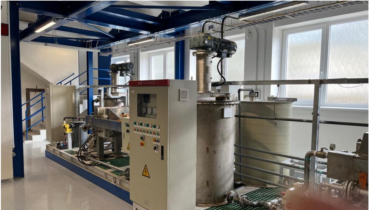
**Photo 7. HPEMM Dissolution, Deep Final Purification Module**
