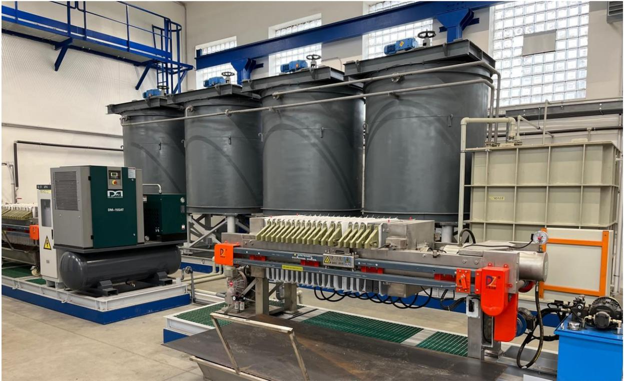
**Photo 3. Post Magnetic Separation: Concentrate and Tailings Tanks and Filter Presses**
