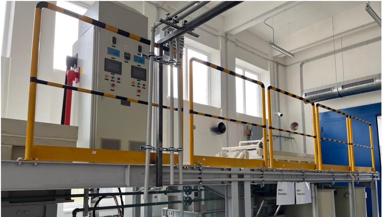
**Photo 6. Electrowinning Module (a purification step in its own right)**
