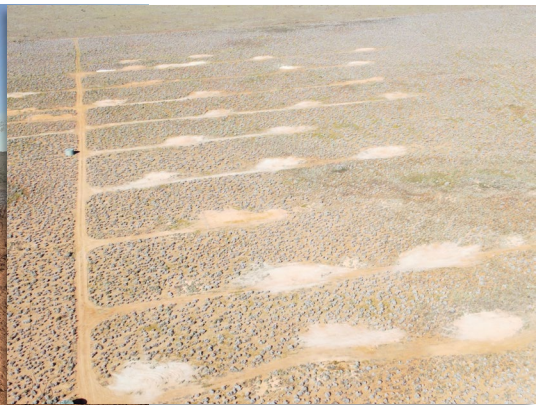
Hydroseeded drillpads
