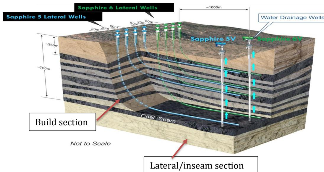
Figure 1: Schematic of Sapphire 5 and 6 pilot well configuration
