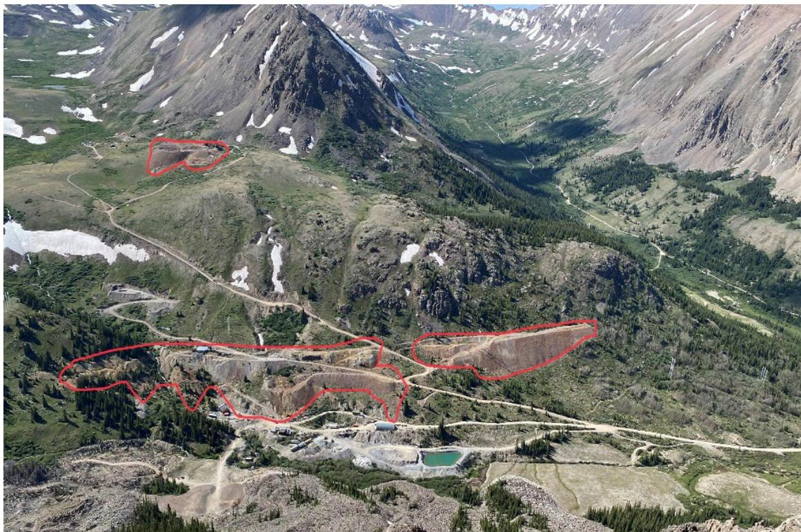
*Figure 2: London mine - surface stockpiles outlined in red*
