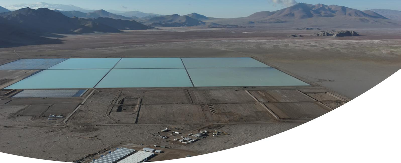
Sal de Vida is designed to produce battery grade lithium carbonate through an evaporation and processing operation located in Catamarca Province, Argentina, approximately 200km from Olaroz. Stage 1 of this project will deliver an initial 15ktpa operation that will be expanded to ~45ktpa through Stage 2.
