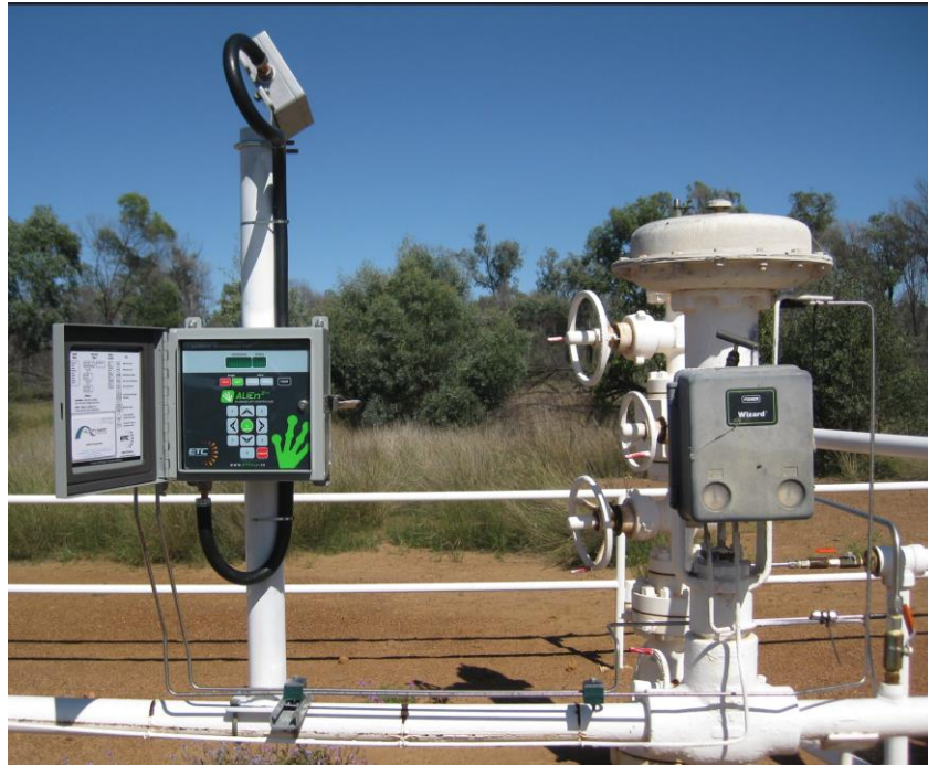
Kincora #40 well site intermitter unit – installed Nov 2022
