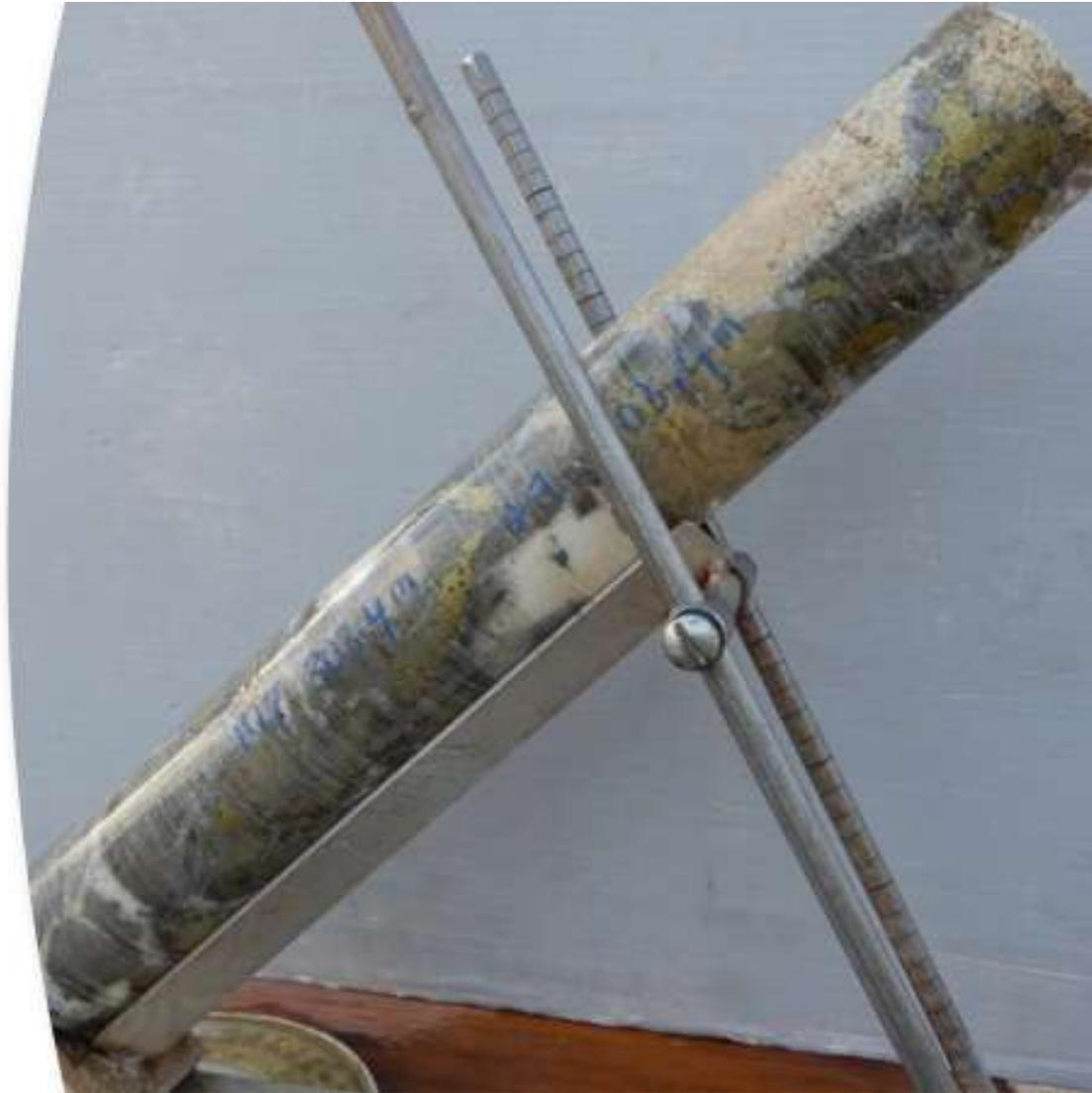
Example of hydrothermal infill breccia at Mt Cannindah from hole 17
