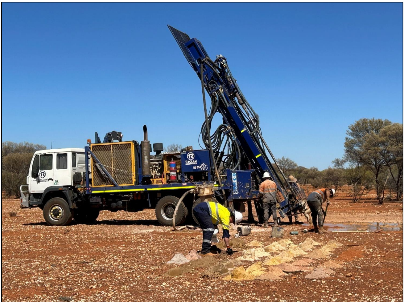
Figure 2 – AC drilling at Gidgee North
