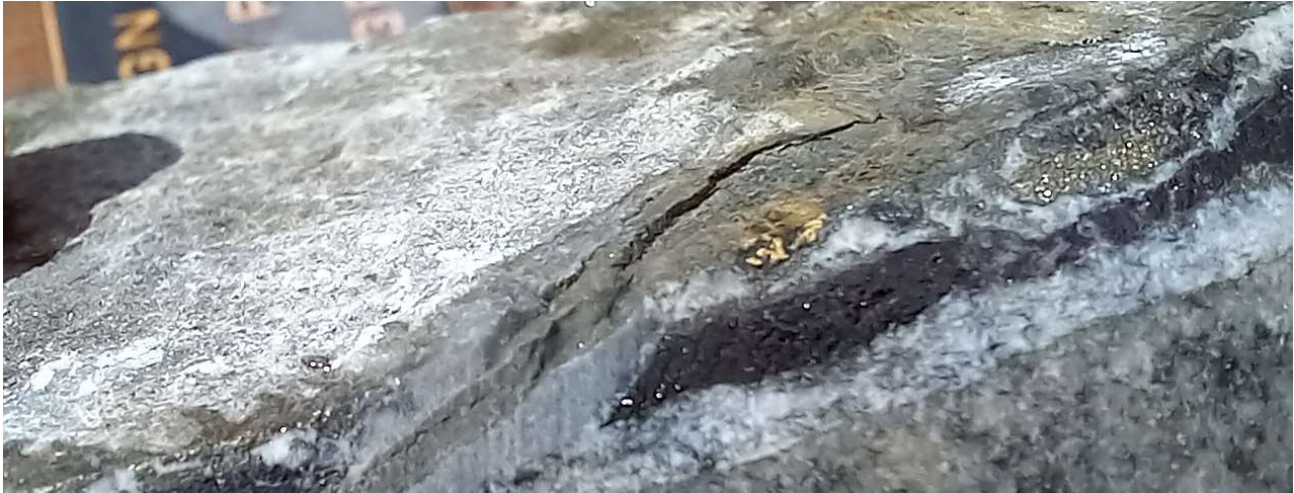
Fig 10 Visible gold in quartz pyrite -black sphalerite vein cutting diorite (centre of photo), Section HQ core, Hole 17 109m-110m returned 1m @ 1.04 g/t Au
