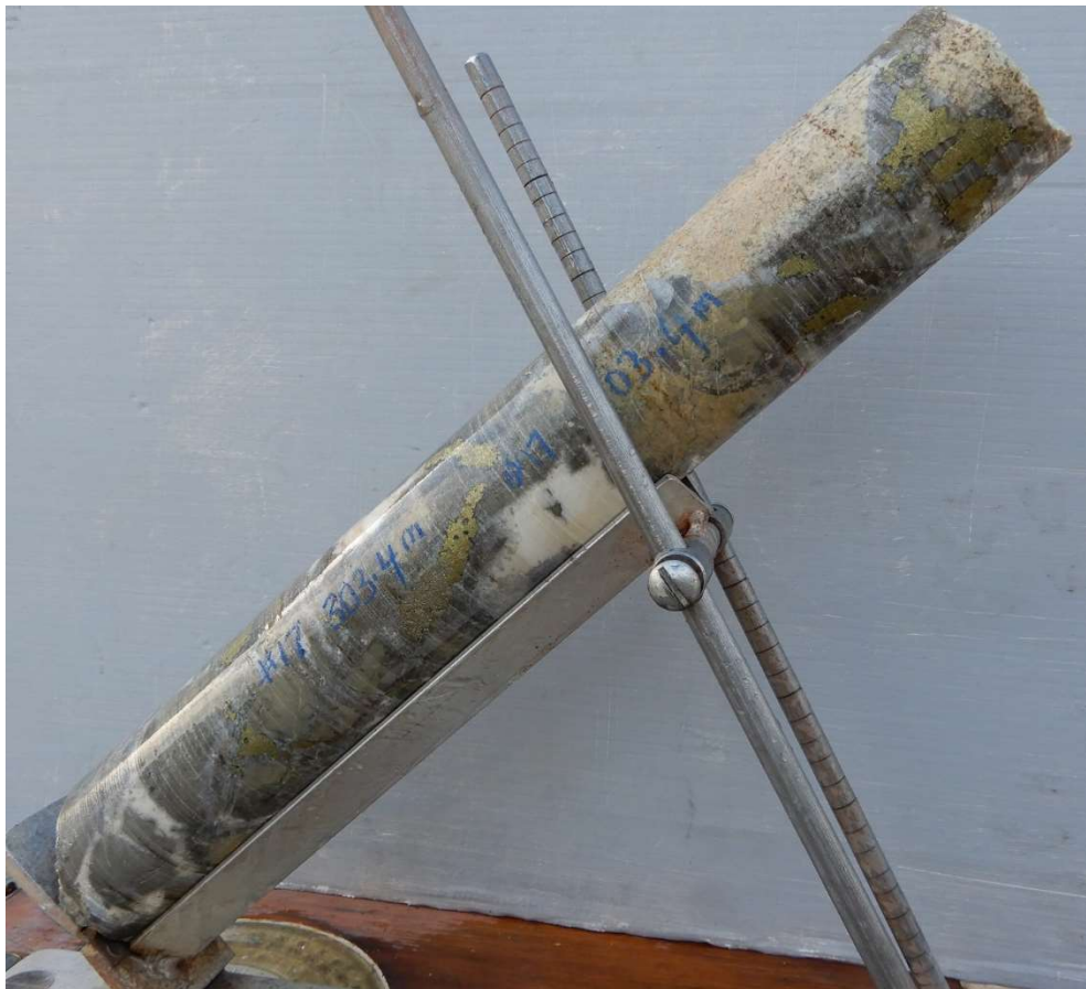
Fig. 11. Photo full HQ core Hole #17 , oriented in core oriented frame, hole drilling to south-south- west , view looking west north west , hole at 303.4m inclined at -44.5 degrees toward 206 degrees mag: Hydrothermal Infill Breccia. Clasts of grey hornfels and light pink carbonate altered (ankeritic) diorite with infill of abundant chalcopyrite (golden) , pyrite (brassy) , calcite (white) , quartz (glassy). Interval 303m to 304m : 1m @ 3.25% Cu, 0.44 g/t Au, 47.1 g/t Ag, 7.12% S. Veins striking east west (262mag) , dipping north -71 degrees. (Dip direction = 352 mag).
