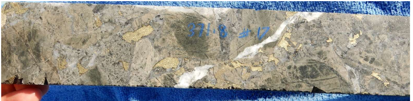
Fig 13. Half HQ Core : Hydrothermal breccia with clasts hornfels, diorite, infill chalcopyrite , pyrite, quartz , calcite, minor chlorite. 371m-372m returned 1m @ 2.1% Cu, 0.32 g/t Au, 16.9 g/t Ag, 2.76% S.
