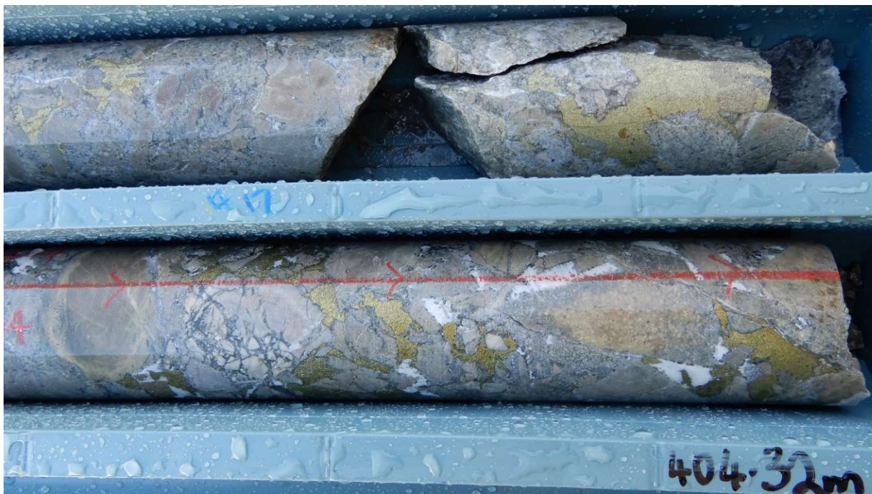
Fig 17 Full HQ Core. Hydrothermal breccia with clasts hornfels and infill chalcopyrite, pyrite, quartz, calcite, minor chlorite. 403m-404m returned 2m @ 1.49% Cu,0.35 g/t Au,15.6 g/t Ag, 1.86% S.
