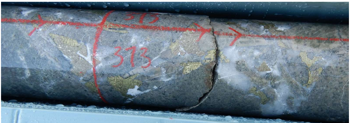
Fig 14. Full HQ Core. Hydrothermal breccia with clasts diorite and infill chalcopyrite, pyrite, quartz and calcite. 372m-374m returned 2m @ 1.49% Cu, 0.30 g/t Au, 14.1 g/t Ag, 5.54% S.
