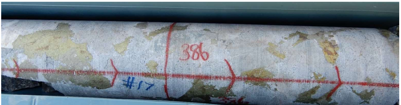
Fig 16 Full HQ Core : Hydrothermal breccia with clasts hornfels, diorite, infill chalcopyrite , pyrite, quartz ,calcite, minor chlorite. 386m-388m returned 2m @ 1.21% Cu,0.12 g/t Au,10.6 g/t Ag, 2.59% S.
