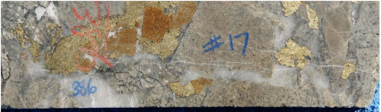
Fig 15 Half HQ Core : Hydrothermal breccia with clasts hornfels, diorite, infill chalcopyrite , pyrite, quartz ,calcite, minor chlorite. 386m-388m returned 2m @ 1.21% Cu,0.12 g/t Au,10.6 g/t Ag, 2.59% S.
