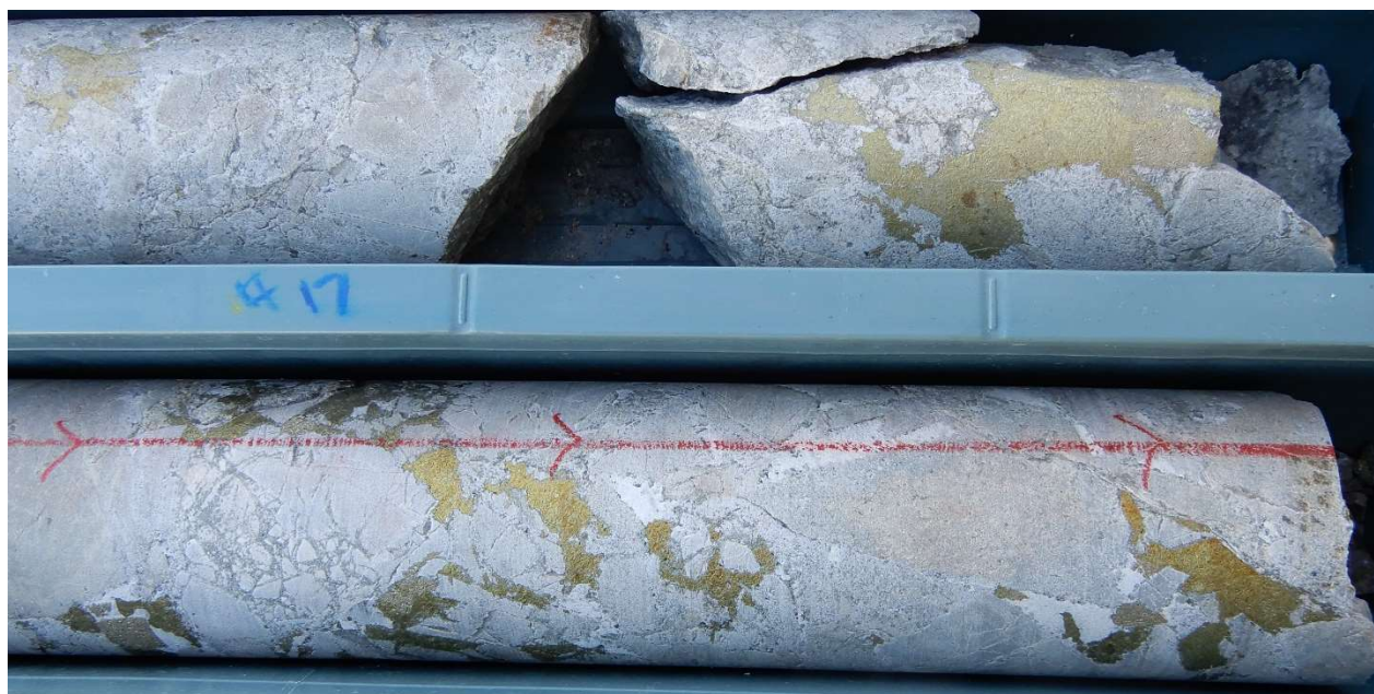
High grade copper in hydrothermal infill breccia CAE hole # 17: 404m depth. Interval 404m-407 : 3m @ 1.85% CuEq*, 1.52% Cu ,0.31 g/t Au,17.2 g/t Ag.
