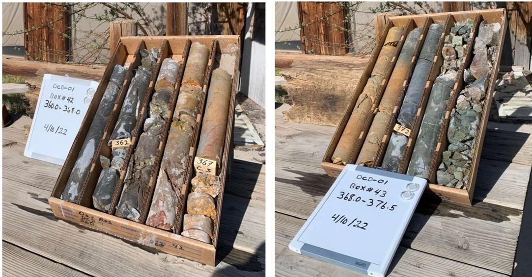
Figure 8: Altered and mineralised target zone intersected in DCD-01
