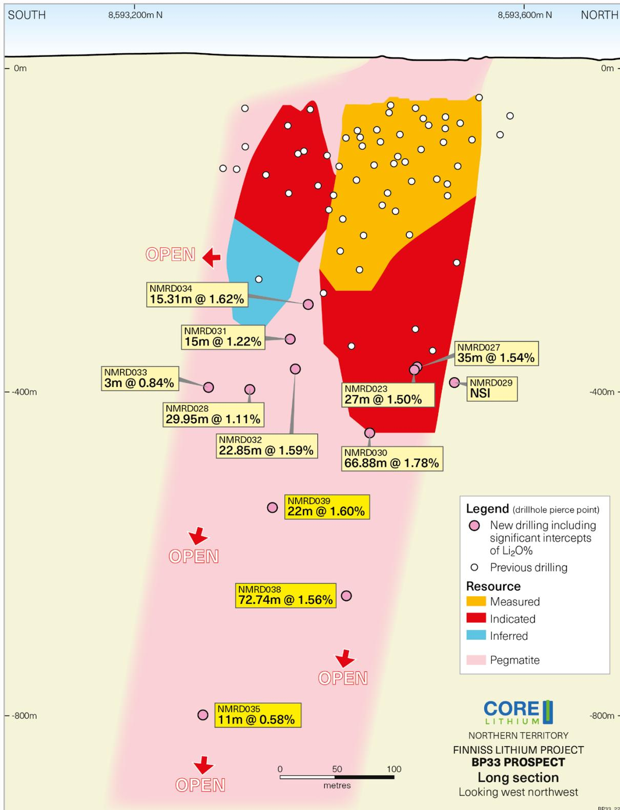
Figure 1. Long-section for BP33 showing the current Mineral Resource (coloured by resource category), with new assay results included (intercept widths are not true width).
