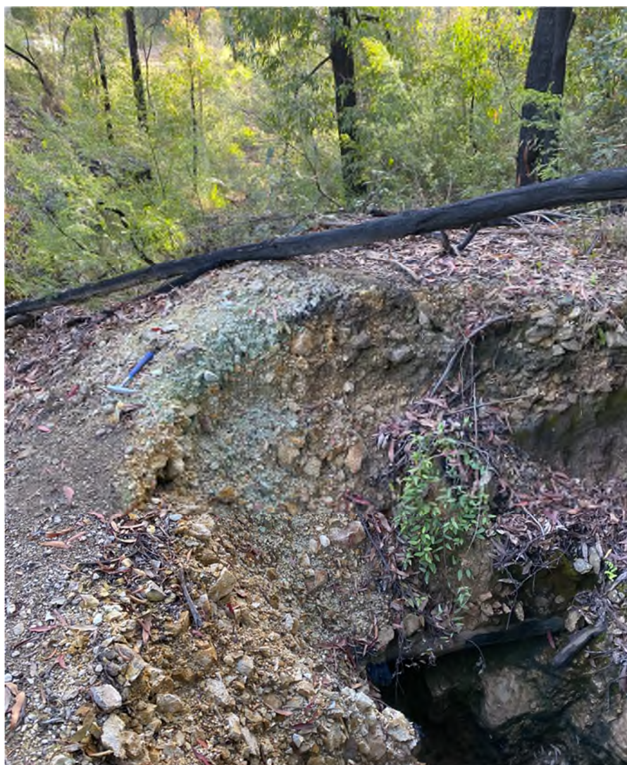
Figure 5: Historic working noted on Figure 2 south of Kylo Pit with malachite in the mullock during recent Thomson Resources field trip
