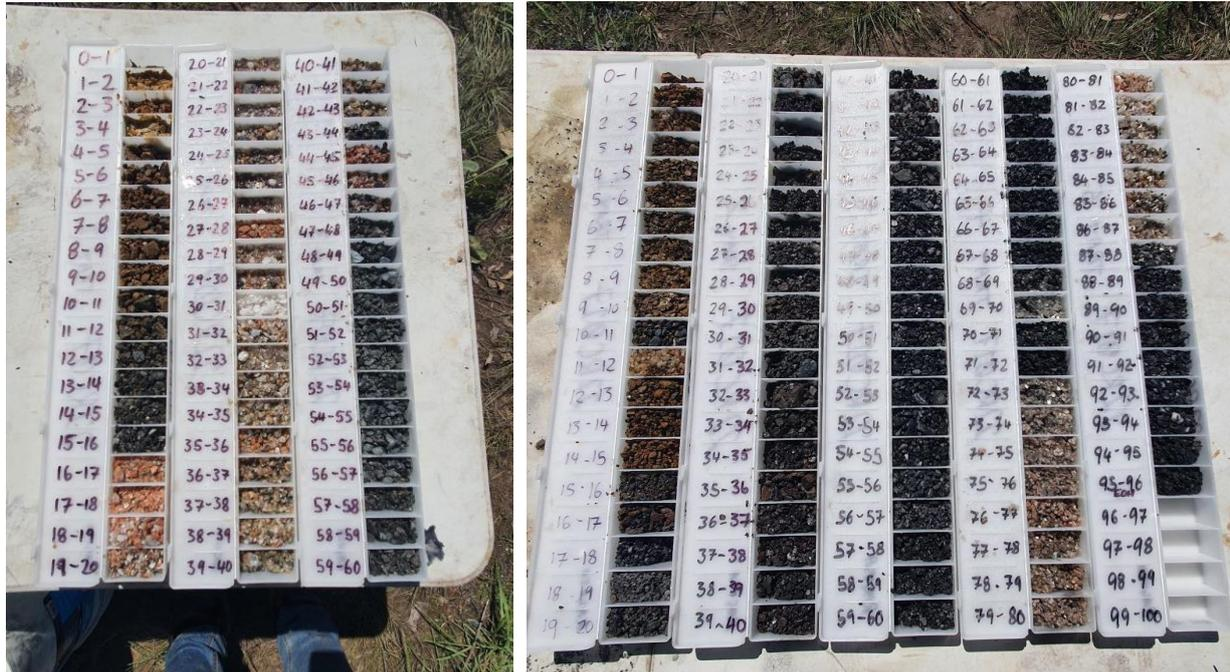
**Figures 1-2. RC Drill Chips – Drillhole 22RC07 (Pegmatite 16m-43m) (L) & Drillhole 22RC017 (Pegmatite 72m-87m) (R)**
