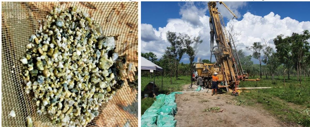
**Figures 3-4. RC Drill Chips with apple-green minerals (L) & RC Drilling Operations (R)**
