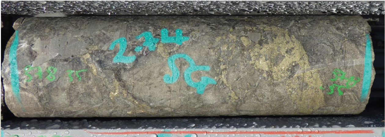
Figure 4: Drill core from WFDH375 378.7 metres showing chalcopyrite as matrix infill in the Walford Dolomite (sample is roughly 40 m from the Fish River Fault)
