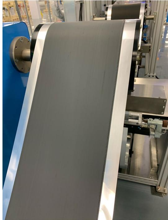
**Figure 3 & 4: Cathode slurry mix and cathode production from iM3NY factory floor**
