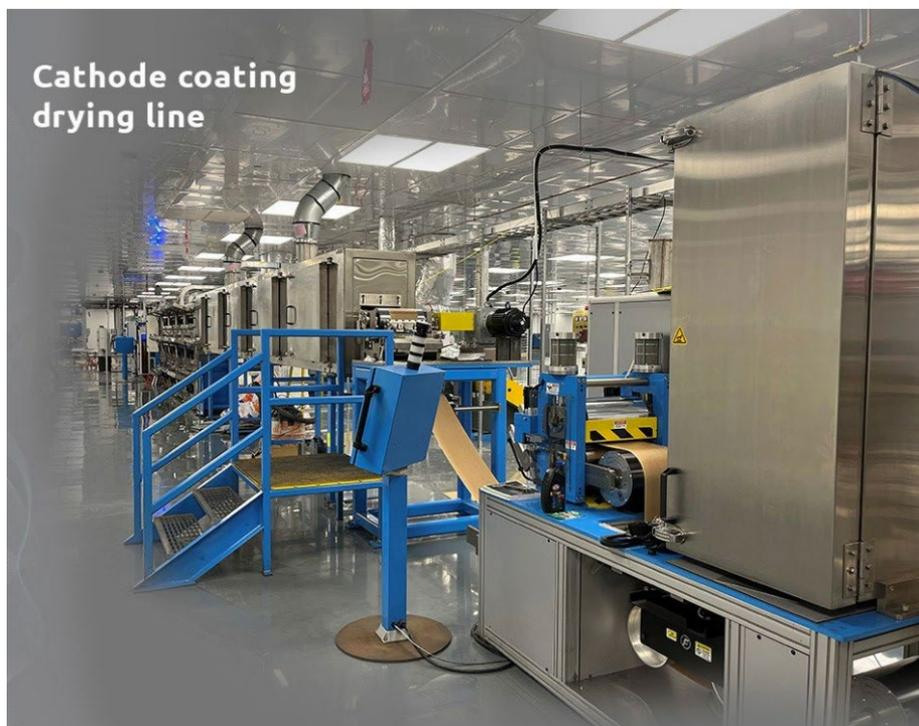
**Figure 5: Cathode Coating Drying Line**
