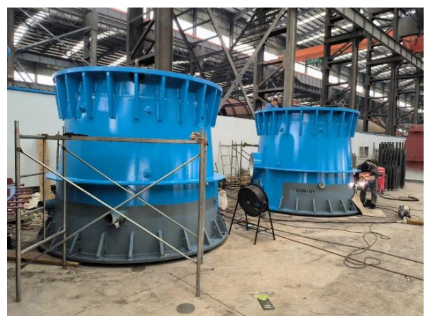
Figure 5: Andritz, Draft Tube Cone - September 2022
