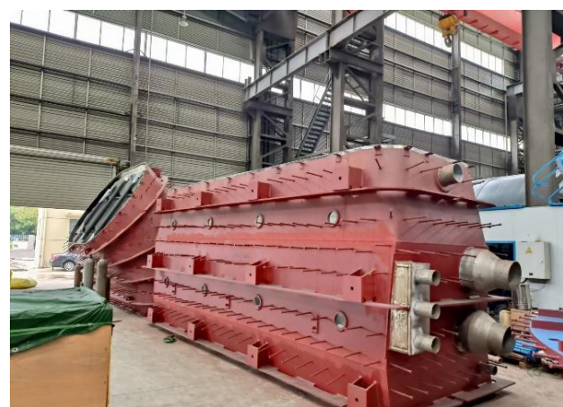
Figure 4: Andritz, Draft Tube Liner - September 2022
