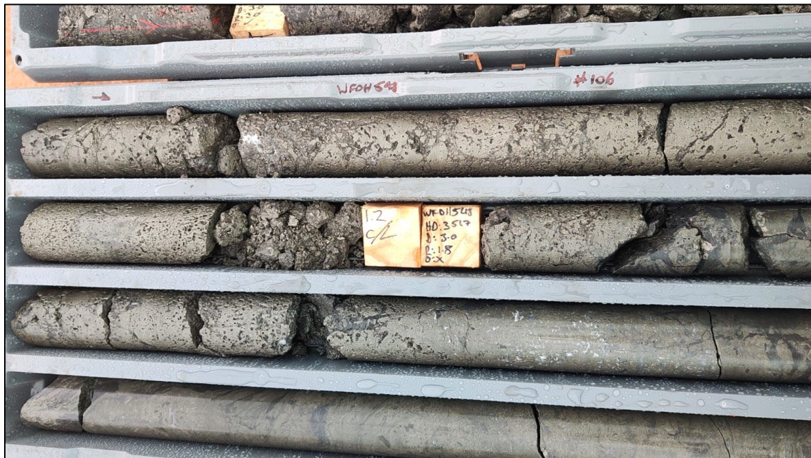
Figures 8: Drill core from WFDH548 showing massive to breccia replacement sulphide mineralisation at Amy West
