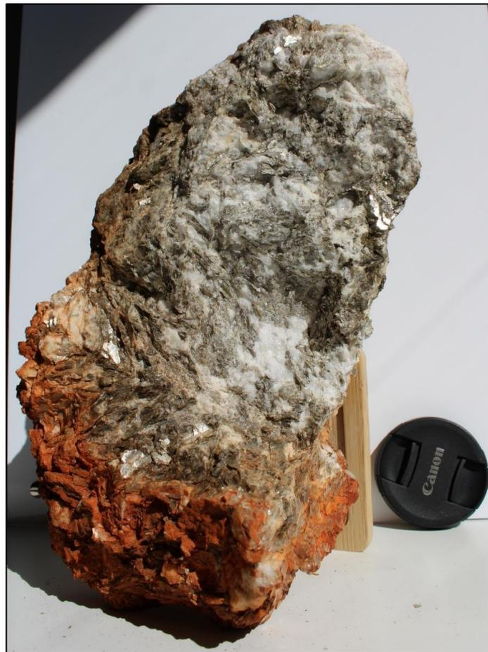
**Figure 8** – Sample of Mica portion of fractionated pegmatite
