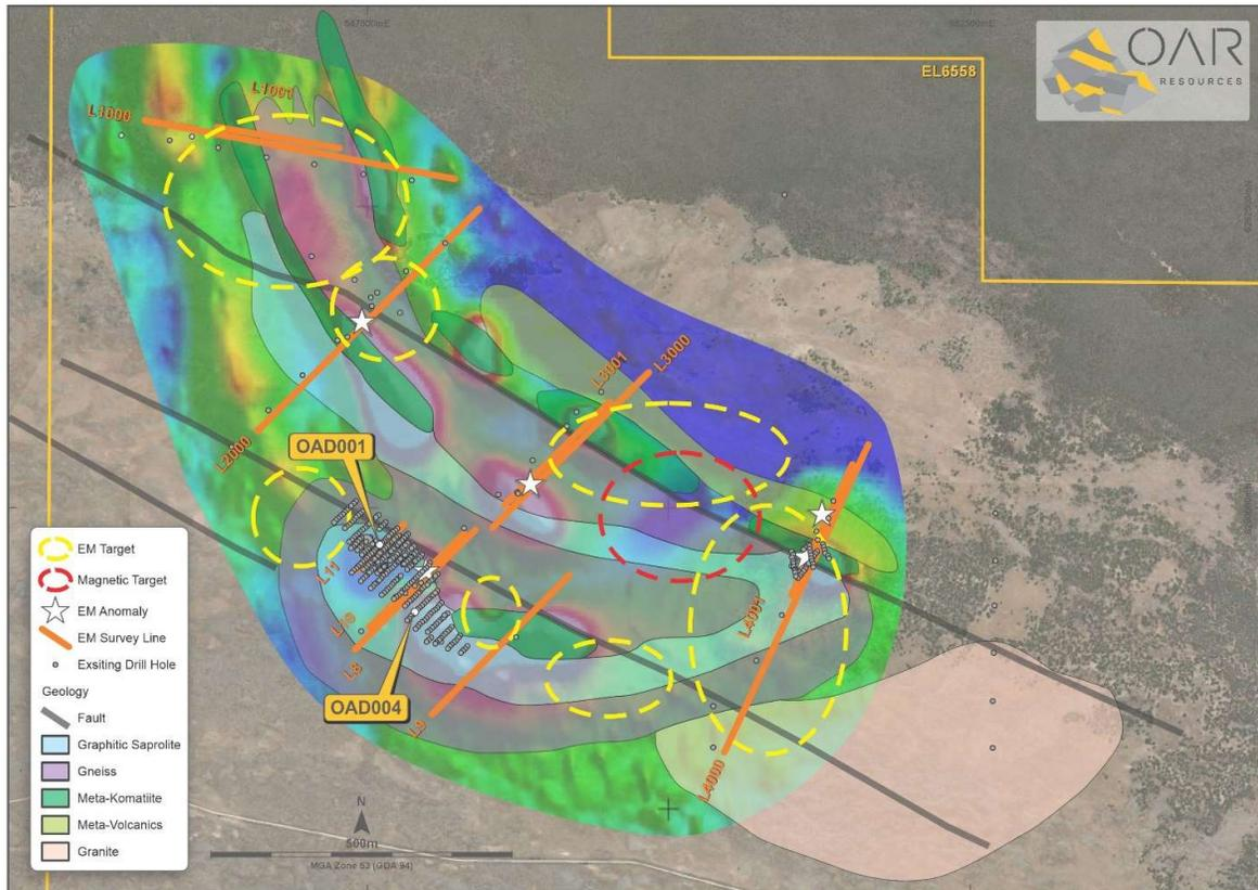
Figure 2: Interpreted geophysical targets with locations of holes sent for metallurgical test work
