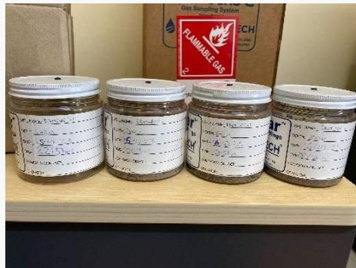
Mudgas samples from different levels, awaiting testing
