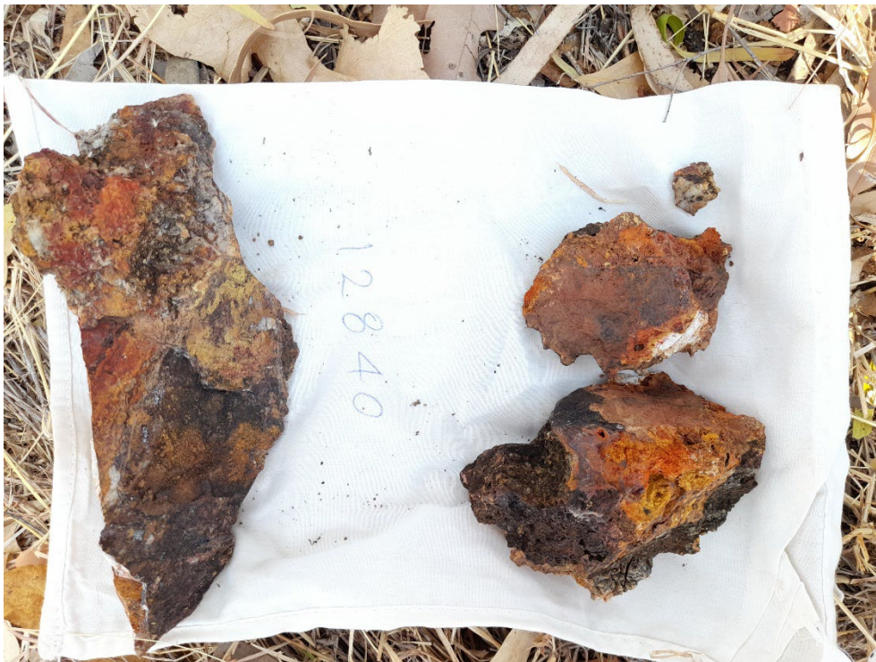
PLATE 2: Sample 12840, of mullock from shallow pit west of the main Pinnacles workings, composed of vuggy quartz vein material with limonite boxworks after sulphides (11.95 g/t gold).
