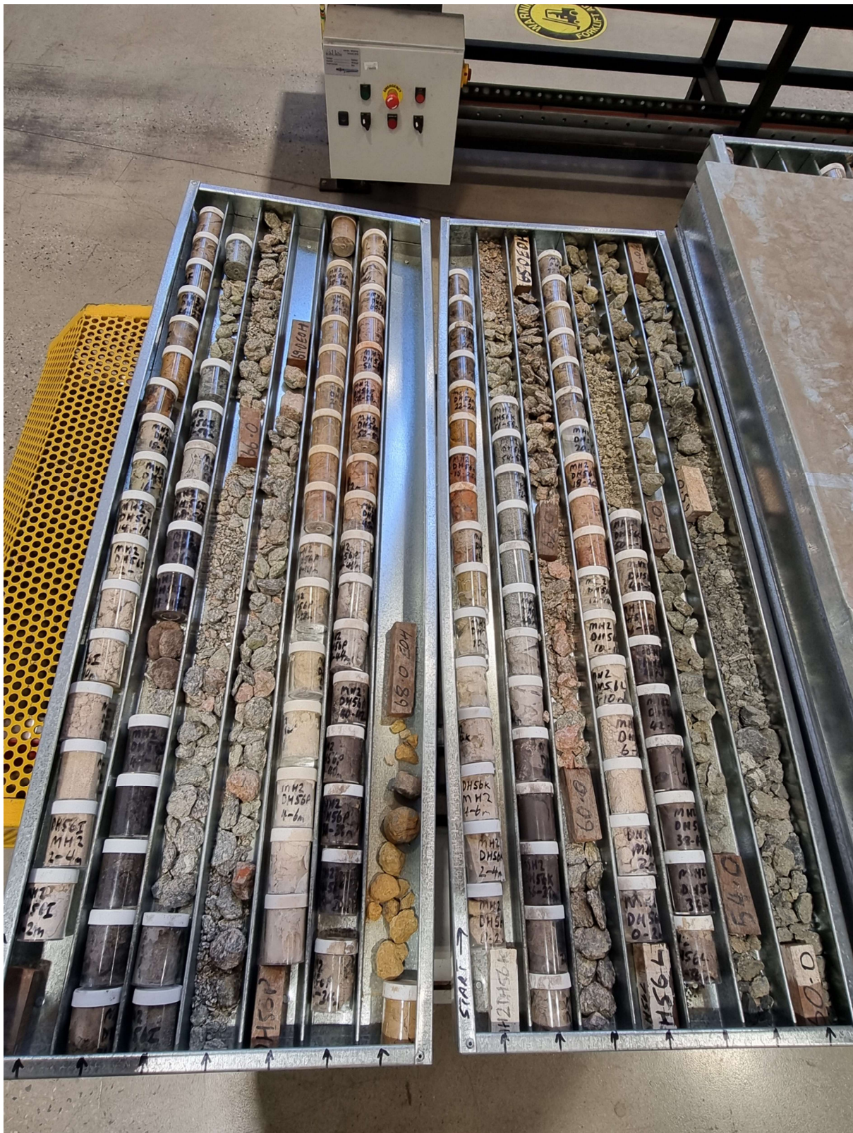
Figure 6. Example of aircore drilling samples and bottom of hole samples, which are available for re-sampling at DEM's exploration library.
