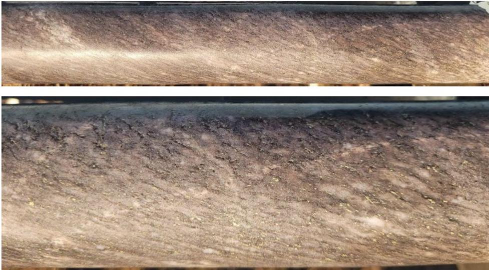
Figure 3. Quartz diorite porphyry with quartz eyes, showing strong secondary silica and biotite alteration and strong chalcopyrite mineralisation along the foliation (CCDD003, 140.5m).
