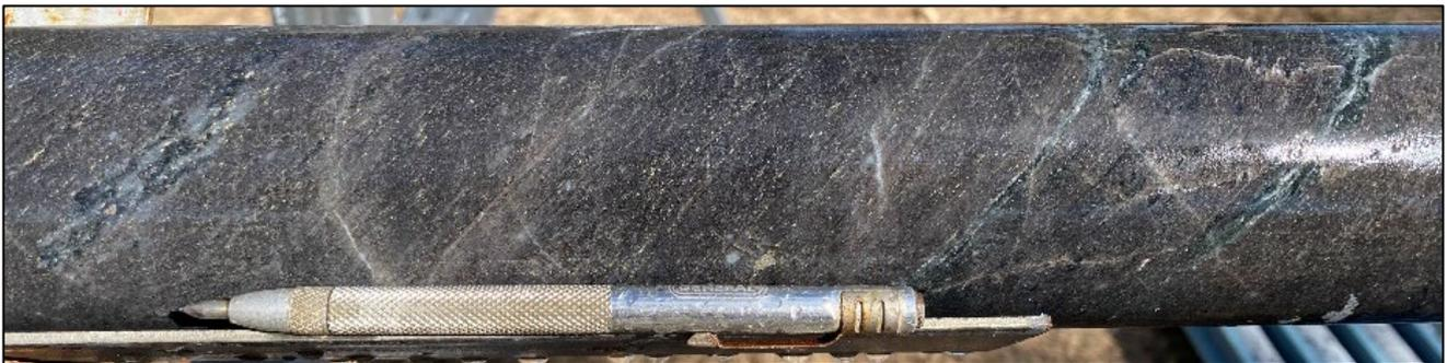
Figure 9. Quartz diorite with chalcopyrite and pyrite mineralisation along foliation, with strong biotite and minor chlorite alteration (CCDD001, 64m).
