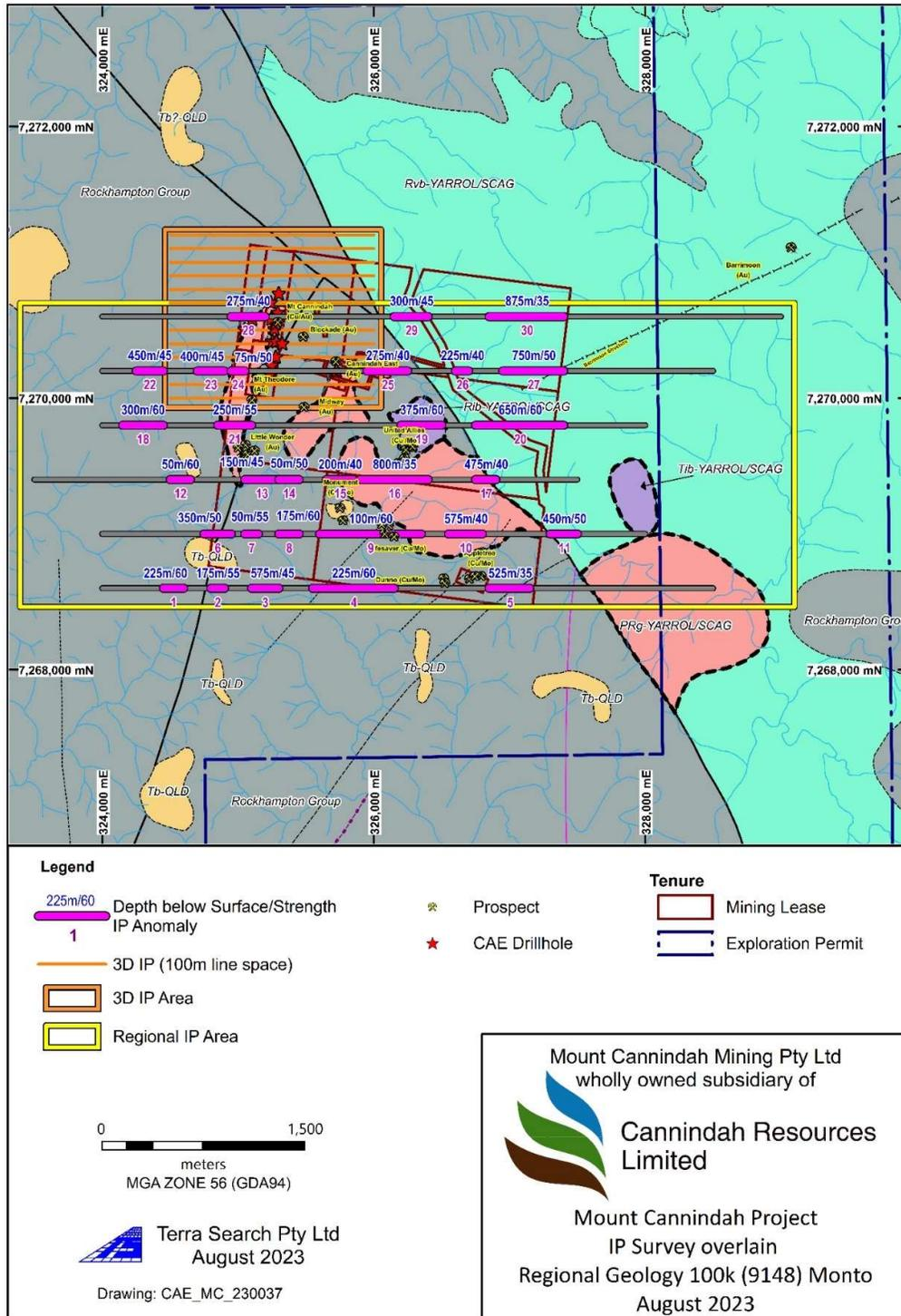
Fig 8. Mt Cannindah, Aug 2023 MIMDAS IP Survey. Location of 30 x IP Chargeability anomalies taken from the Inverted Cross sections and presented in plan view on the published geology base. Each IP anomaly annotated with depth from surface to central position of anomaly in metres and intensity of chargeability anomaly in mV/V.
