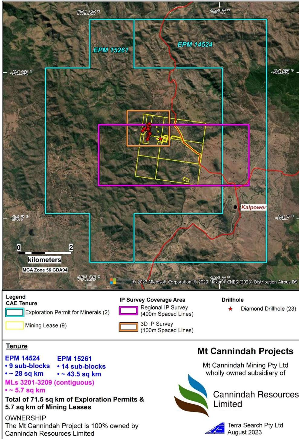
Fig 2. Cannindah Project CAE 2023 IP survey areas in relation to CAE MLs & EPMs, background is satellite image . Note Regional 400m line spaced regional coverage (approx. 11.25km<sup>2</sup>) & more detailed 3D 100m line spaced survey (1 km<sup>2</sup>). CAE drillholes plotted.
