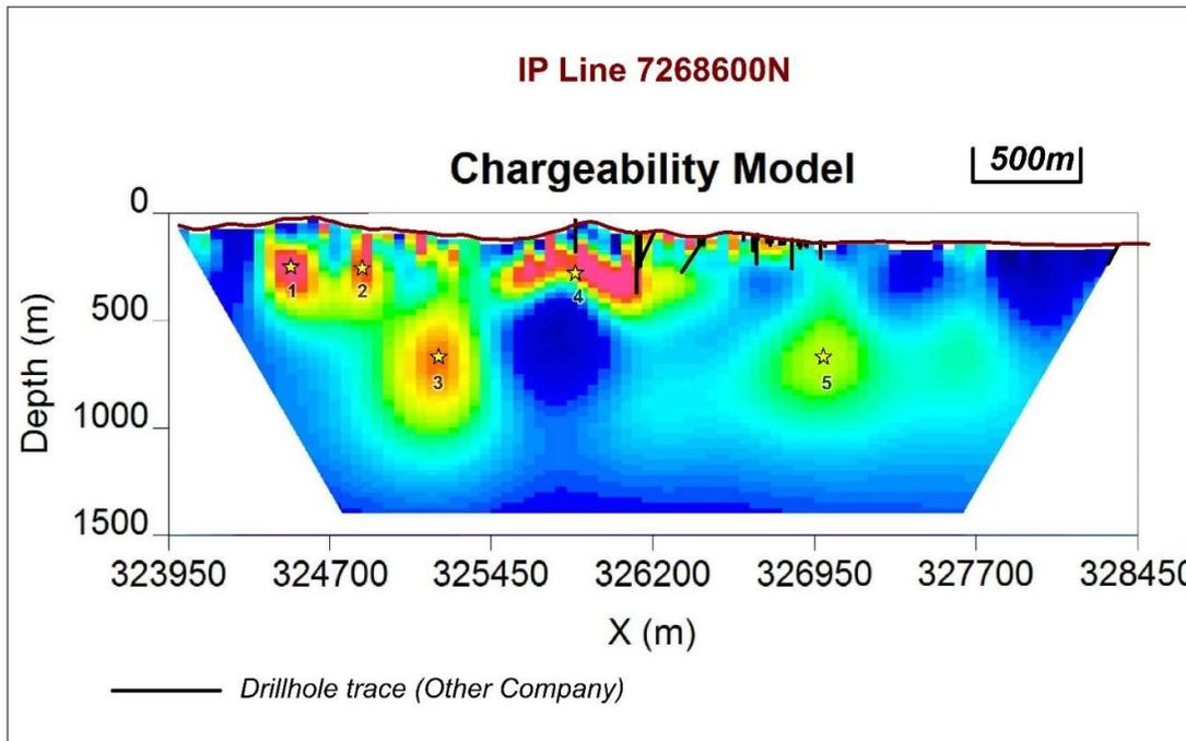
Fig 5. Mt Cannindah, Aug 2023 MIMDAS IP Survey. Preliminary Chargeability Inversion Model Images. Regional Survey Lines (a) 7269000N : over SW IP anomalies & Lifesaver Cu-Mo Prospects (b) , 7268600N over SW IP anomalies & Lifesaver South Cu-Mo Prospects, Dunno & Appletree magnetite skarns and deeper IP target to east. ( GRS Modelling.. Note 500m scale and CAE and other company Drilling. See Fig 3 & 4 for Line & Anomaly Locations)
