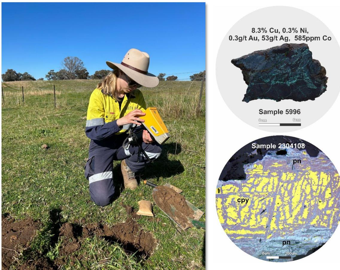
**Figure 7:** Earth AI field team conducting soil sampling at Fontenoy (left), and rock sample 5996 (top right), and nickel sulphides (pn - pentlandite), copper sulphides (cpy - chalcopyrite) confirmed in serpentinite/gabbro through SEM and petrographic analysis (bottom right).
