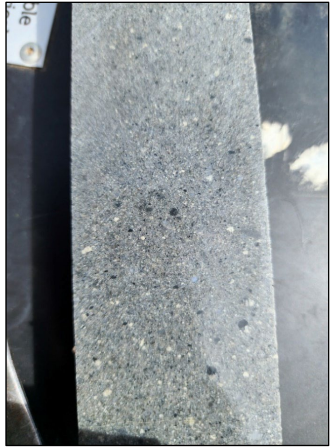
Figure 9: Massive sandstone with blebs of sphalerite MPD005 (274.2m)
