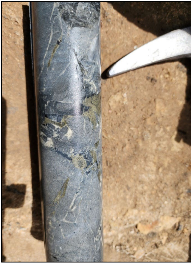
Figure 8: MPD005 core showing brecciation & pyrite infill (268.3m)
