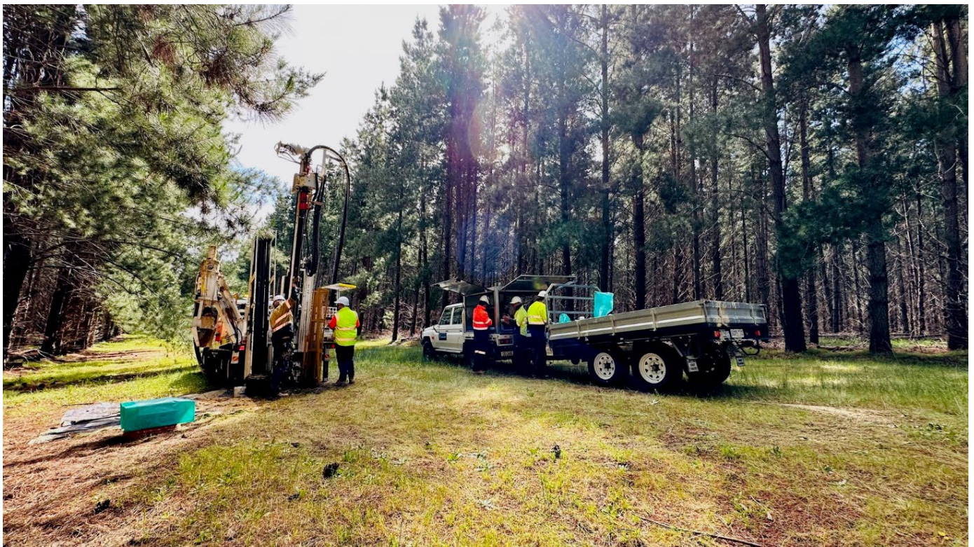
Figure 1- Koppamurra aircore drilling, October 2023.
