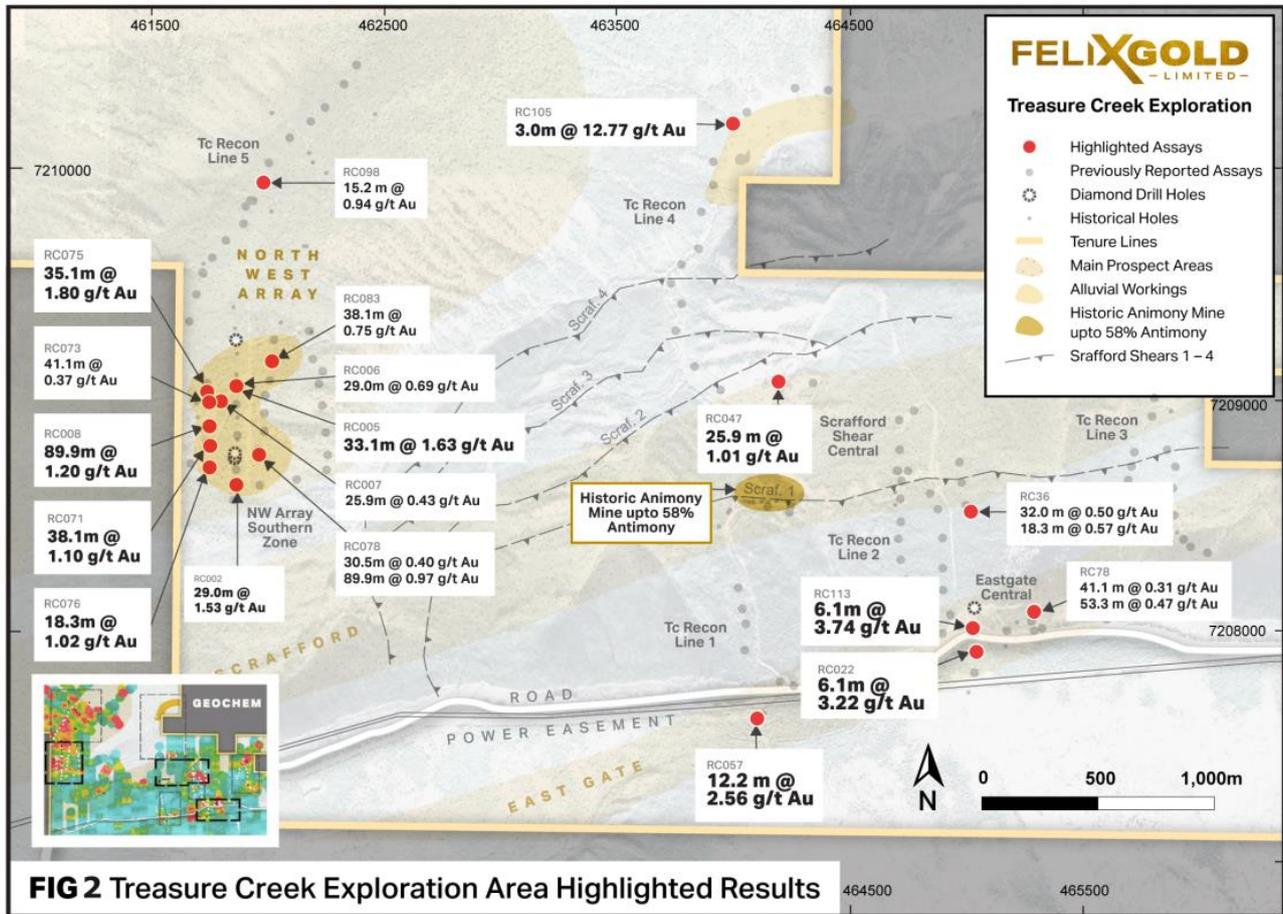
Results from our NW Array prospect at Treasure Creek delivered multiple thick near surface gold intercepts including 22TCRC008 89.9m @ 1.2 g/t au, 22TCRC005 33.5m @ 1.63 g/t Au, 22TCRC071 38.12m @ 1.1 g/t Au, 22TCRC075 35.1 m @ 1.8 g/t Au, and 22TCRC078 89.9 m @ 0.97 g/t Au.
