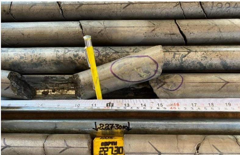
Figure 1 Massive sulphide unit of 4.15m showing sulphide composition and chalcopyrite blebs
