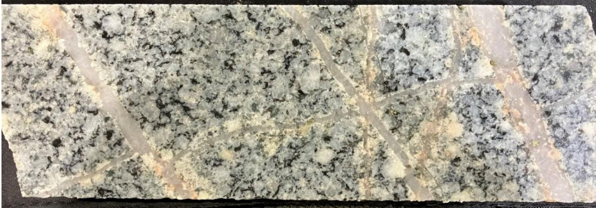
Figure 2 Copper sulphides in mineralised porphyritic granodiorite, Briggs Central. Hole 23BRD0016 at 123.5m, within a 2m interval of 61mm diameter core which assayed 0.31% Cu.
