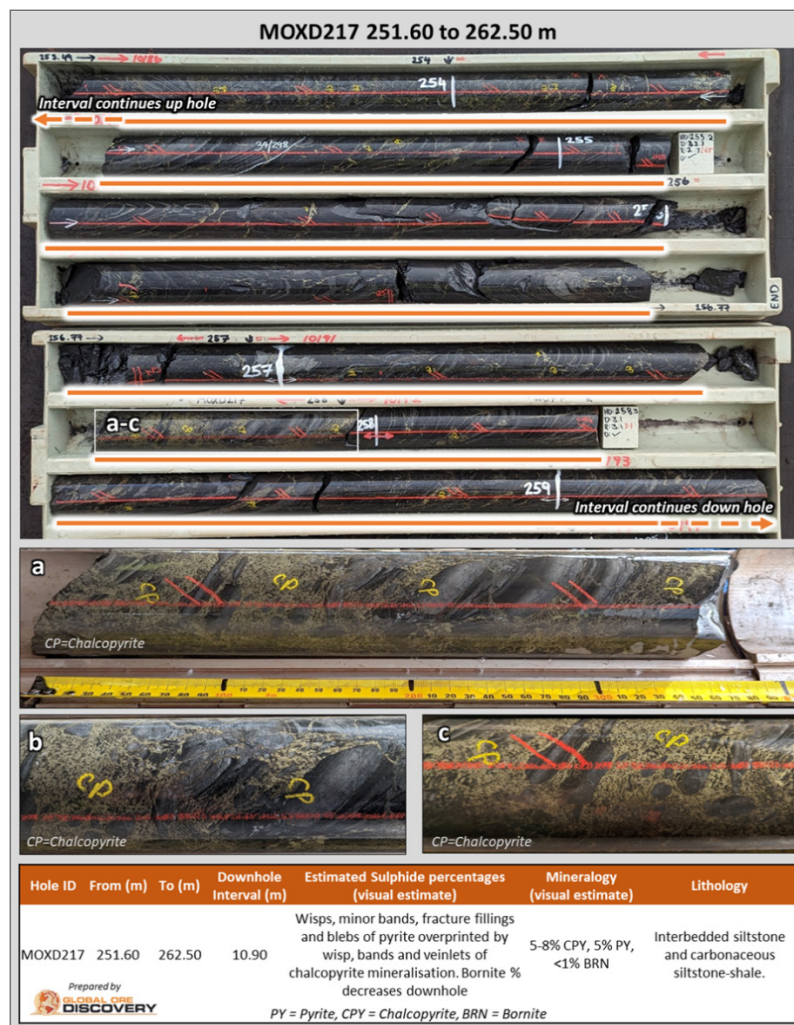
Figure 2: MOXD217 251.6-262.5m 10.9 m wide zone containing wisps, minor bands, fracture fillings and blebs of pyrite overprinted by wispy, bands and veinlets of chalcopyrite mineralisation. Bornite percentage decreases downhole. (a) 257.60 -257.96m strong chalcopyrite infill veining overprint pyrite infill of brecciated siltstone. (b & c) MOXD217 – close ups of chalcopyrite infill veining in brecciated siltstone.
