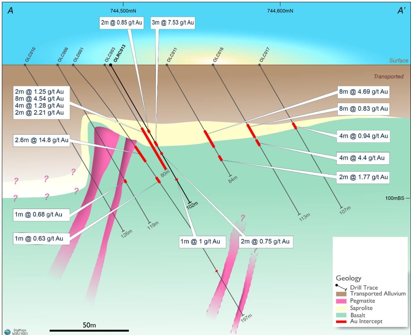
**Figure 2 – Cross Section Showing Historical Drilling and OLRC013**
