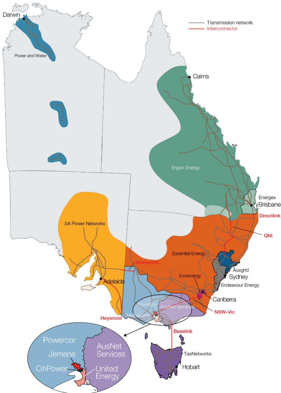
Note: QNI is the Queensland–NSW Interconnector. The AER does not regulate the Basslink Interconnector.
