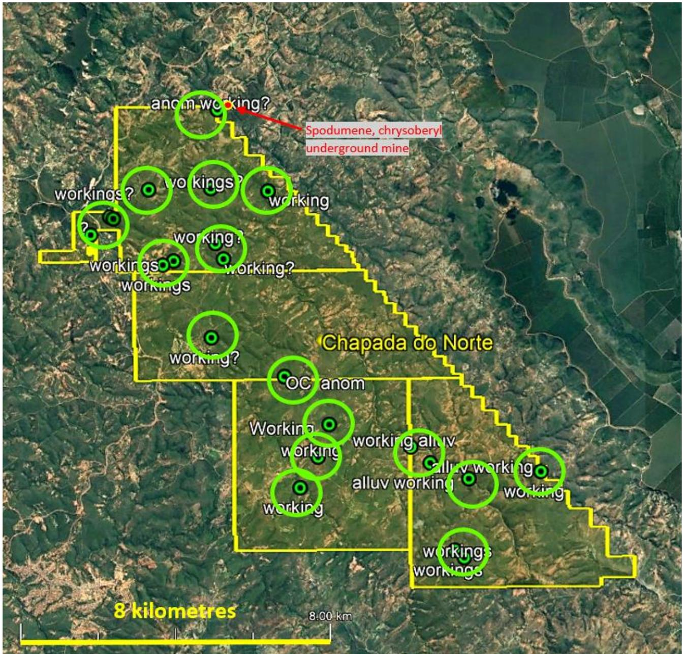
Figure 7. Chapada do Norte satellite imagery anomalies for checking. Note the mine adjacent to the tenements at the NE corner of the current applications.
