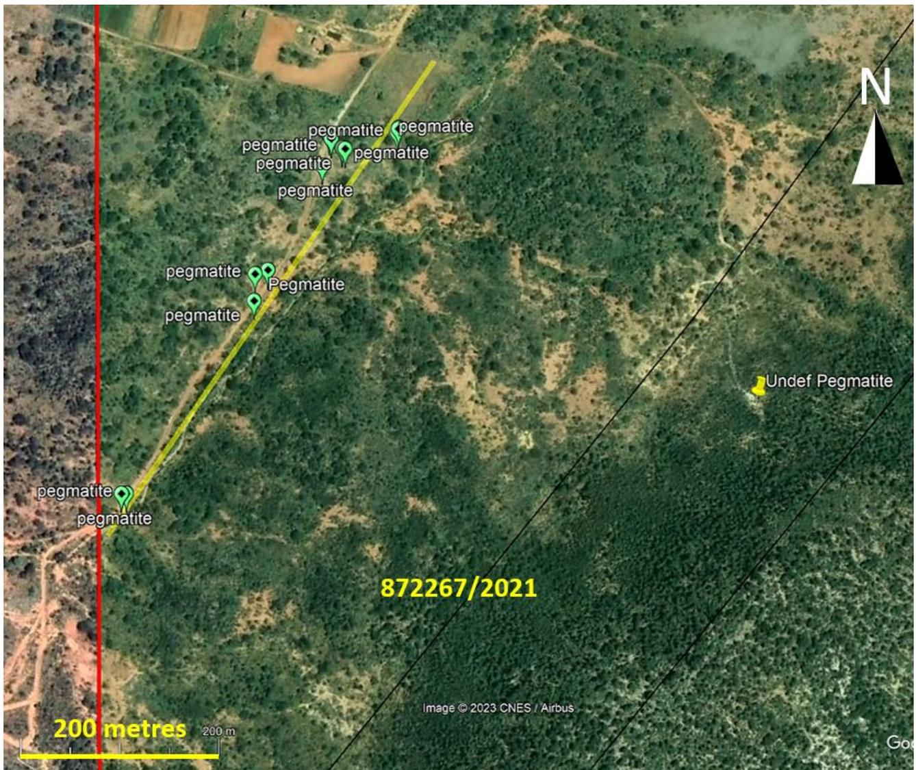
**Figure 4.** Detailed locations of the pegmatite occurrences in 872267/2021 and interpreted strike direction in yellow. Pegmatites with green icon are deformed and with yellow icon an undeformed pegmatite and artisanal working.
