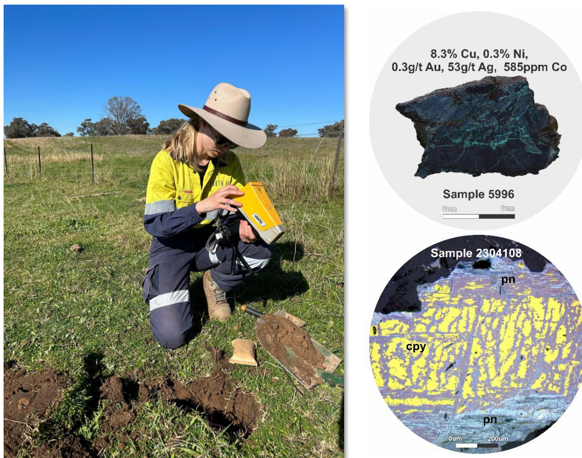
Figure 1: Earth AI field team conducting soil sampling at Fontenoy (left), and rock sample 5996 (top right), and nickel sulphides (pn - pentlandite), copper sulphides (cpy - chalcopyrite) confirmed in serpentinite/gabbro through SEM and petrographic analysis (bottom right).
