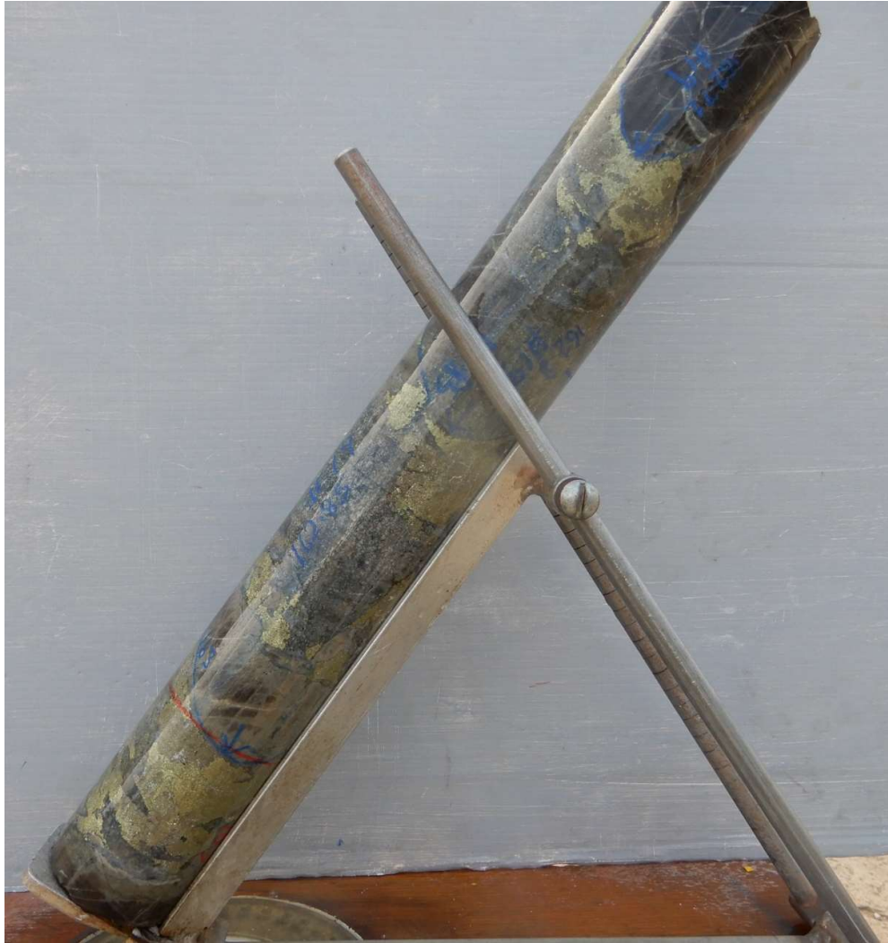
Fig 10. Photo - full HQ core Hole #19, oriented in core oriented frame, hole drilling to south south west , view looking west north west , hole at 163m inclined at -53 degrees toward 217 degrees mag: Hydrothermal Infill Breccia. Clasts of grey, light brown grey hornfels, light grey where sericite altered, minor diorite porphyry clasts with infill of abundant chalcopyrite (golden) , pyrite (brassy) ,minor calcite (white) ,quartz (glassy), dark green chlorite, fine rock flour. 2m interval 162m-164m : 1.64% Cu, 0.39 g/t Au, 20.3 g/t Ag, 6.15% S.
