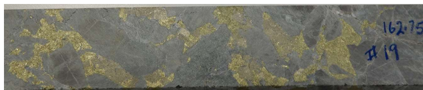
High grade chalcopryrite infill in hydrothermal breccia. CAE Hole 19, 162.5m . 2m interval 162m-164m : 1.64% Cu, 0.39 g/t Au, 20.3 g/t Ag, 6.15% S.
