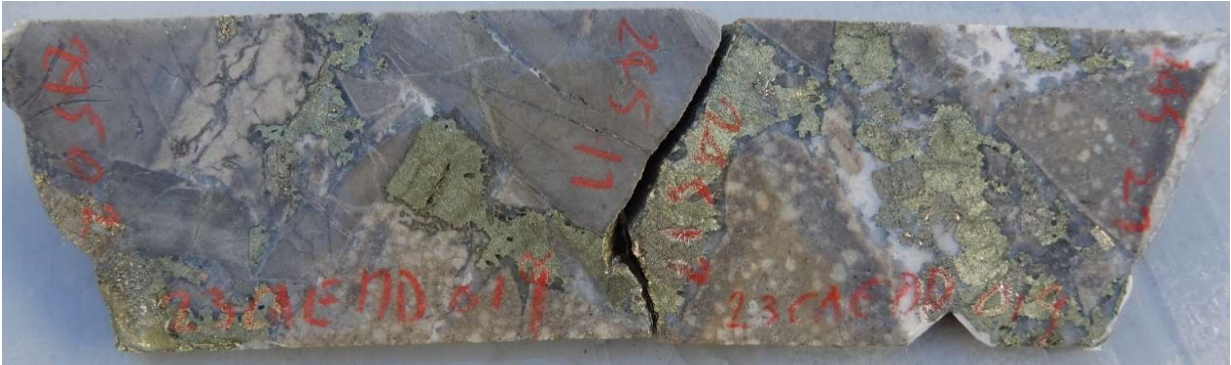
Fig 13. Photo Half HQ Core . Sulphidic hydrothermal breccia at 245m -. Angular clasts grey fine hornfels, feldspar porphyry, infill of golden chalcopyrite, brassy pyrite, white calcite & light grey well formed quartz. 1m Interval 245m-246m grades 1.89%Cu, 1.37 g/t Au, 14.7 g/t Ag, 5.6% S.
