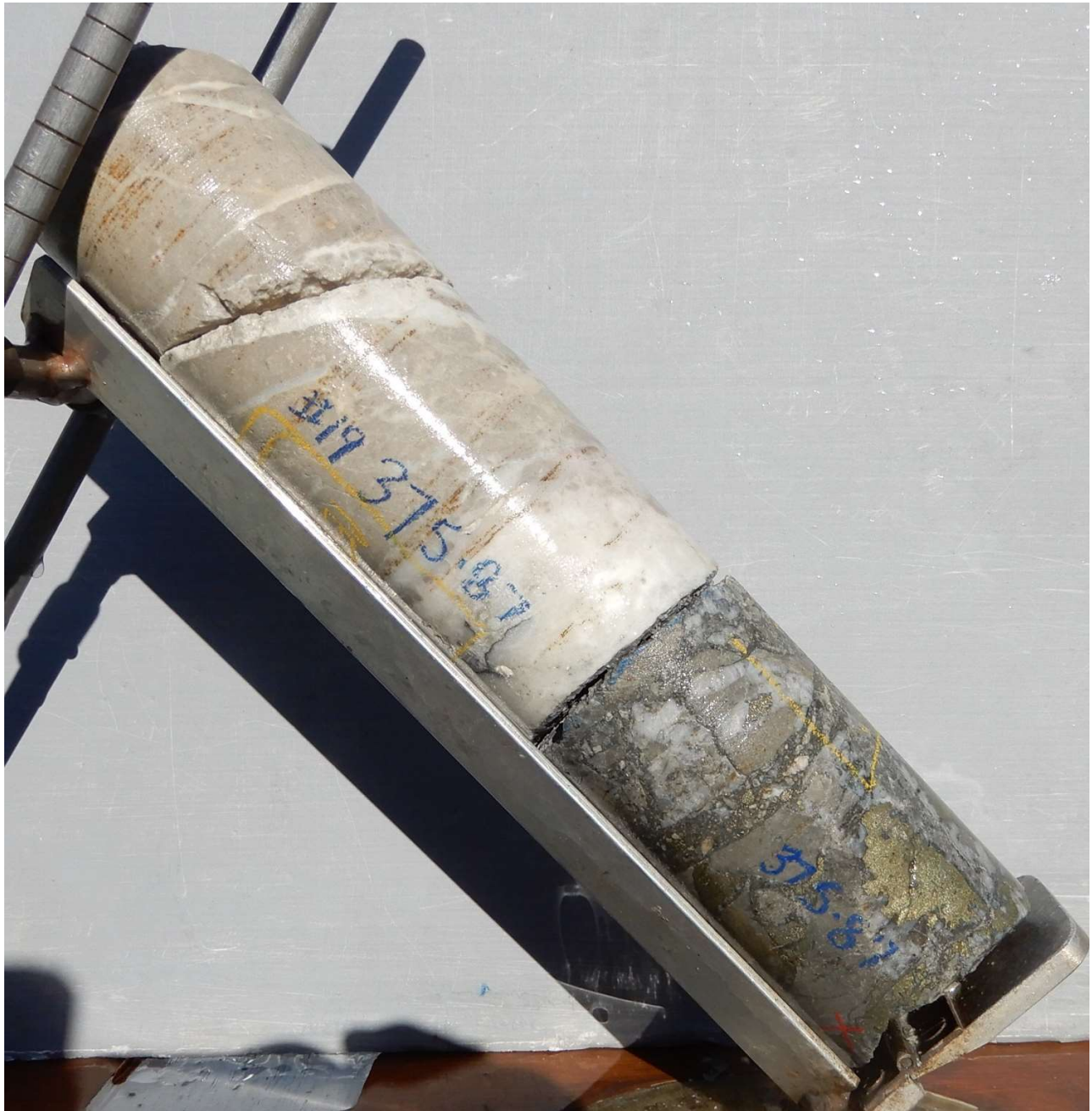
Fig 15. Photo full HQ core Hole #19 , oriented in core oriented frame, hole drilling to south south west , view looking south south west , hole at 375.87m inclined at -46 degrees toward 222 degrees mag: Uphole while , light brown argillised trachyandesite dyke with hydrothermal infill breccia downhole. Clasts dominated by light grey,sericite altered hornfels , with infill of chalcopryrite (golden) , pyrite (brassy) ,minor calcite (white) ,quartz (glassy). 4m Interval 373m-377m grades 0.52%Cu, 1.02 g/t Au, 14 g/t Ag, 6.4% S.
