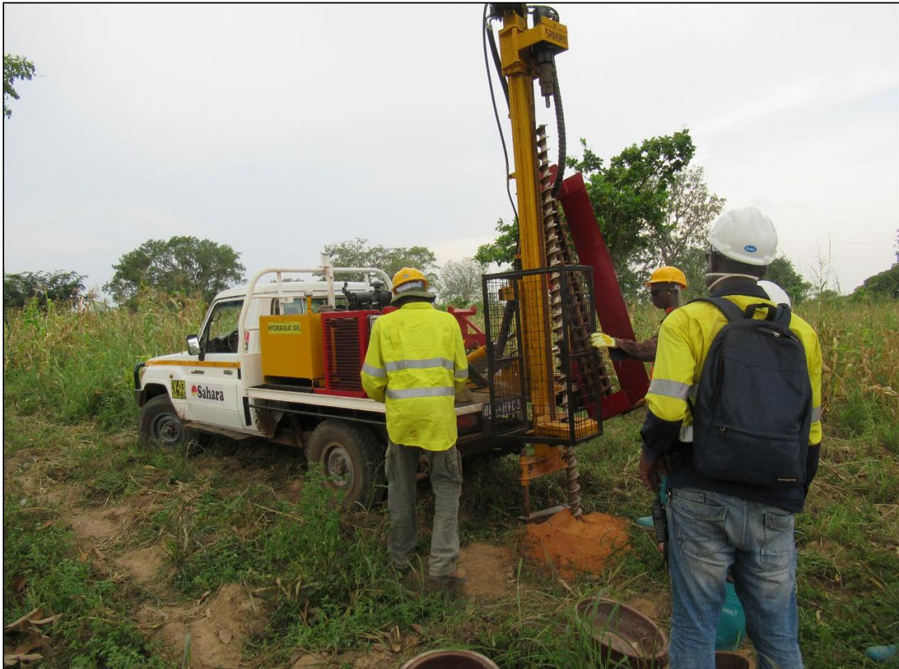
**Figure 2: Auger rig drilling during phase 1 auger program**
