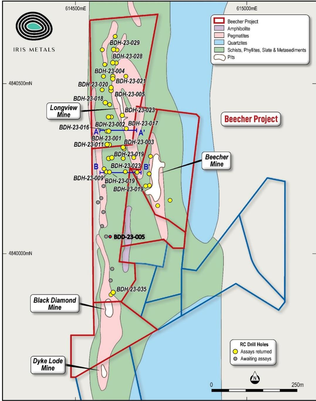
Figure 1: RC drill plan of hole locations.
