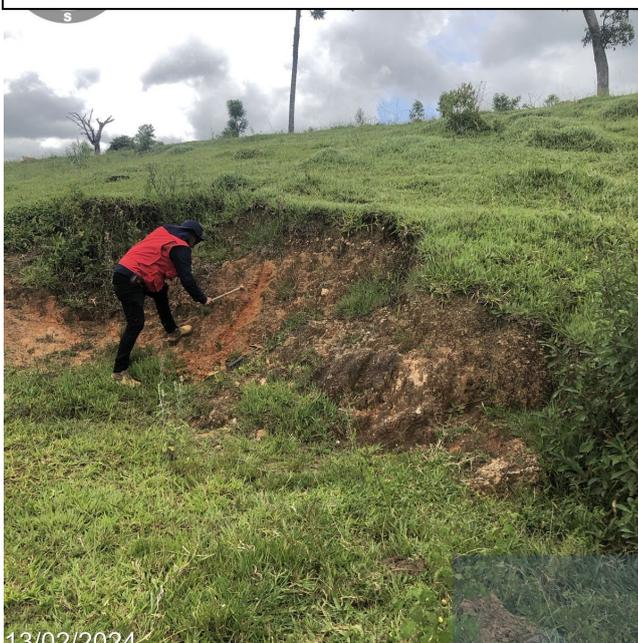
**Photo 4** – mapping and channel sampling saprolite clay
