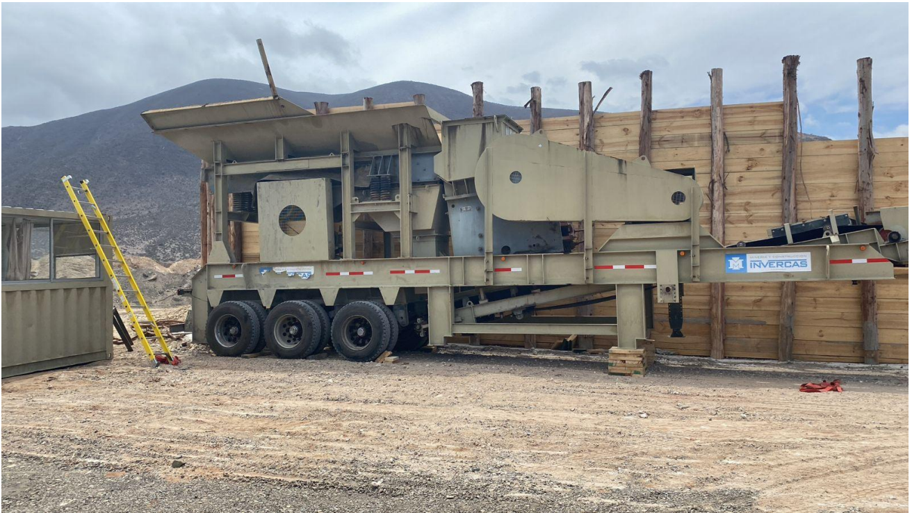
Image 3: Jaw crusher unloaded
