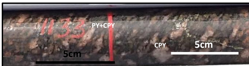
Figure 4: HWDD05 @ 1033m. Fresh gneiss with minor sericite alteration and traces of disseminated pyrite and chalcopyrite (PY+CPY).
