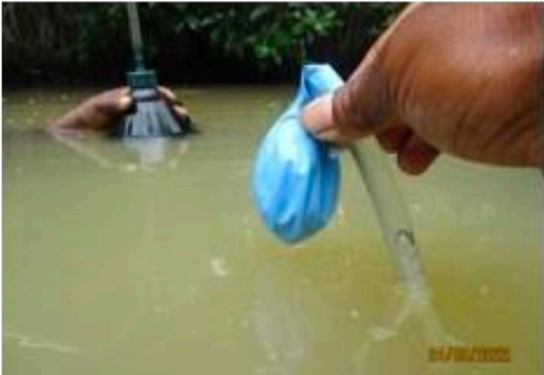
Figure 13: Collection of gas samples at Alligator Creek
