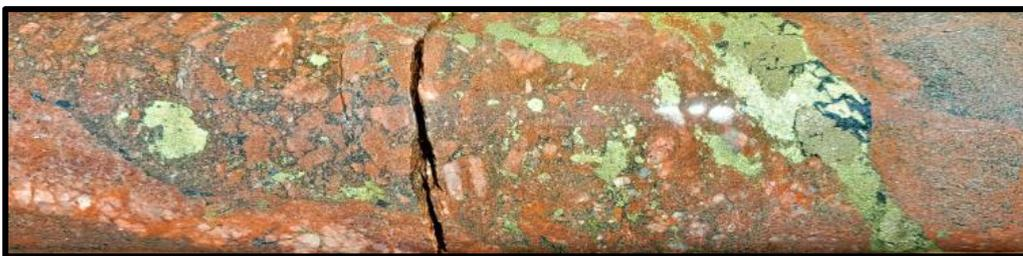
Figure 4: HWDD08 1040.7m 2cm massive chalcopyrite >pyrite-minor magnetite vein, with 5cm magnetite-chalcopyrite-pyrite breccia in footwall.
