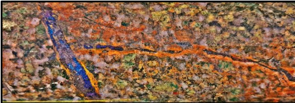
Figure 1: HWDD08 939m Bornite vein with siderite and orange feldspar rim.
