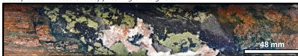
Figure 4: HWDD08 1107.7m 10cm quartz-magnetite-barite-chalcopyrite vein in sedimentary gneiss
