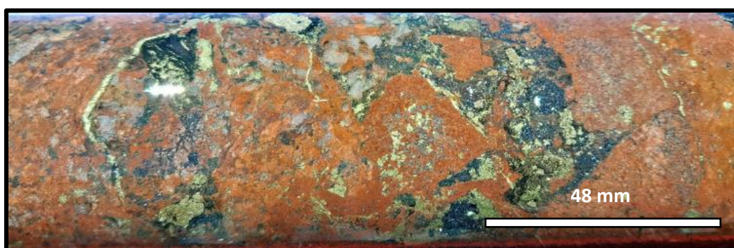
Figure 3: HWDD08 1068.2m Specular haematite-chalcopyrite, chalcopyrite veins, and blebby-disseminated chalcopyrite in granite gneiss.
