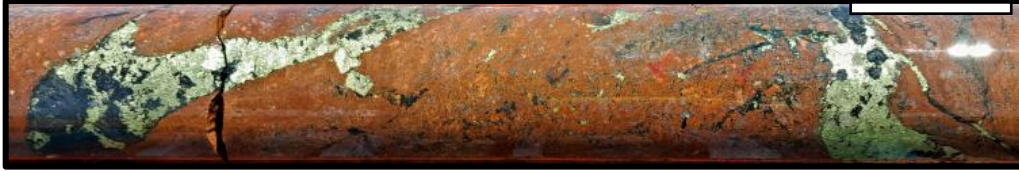
Figure 6: 1135.4-1135.7m Magnetite-chalcopyrite veins in gneiss
