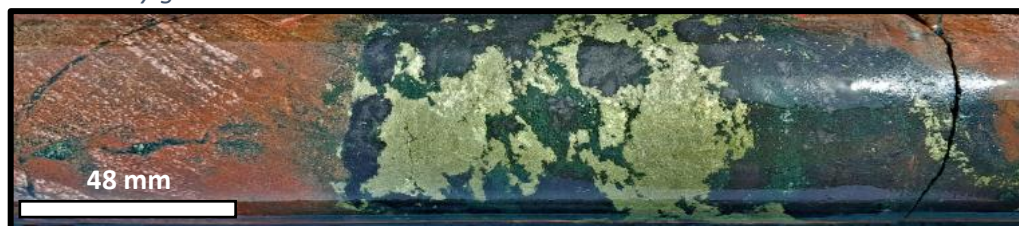
Figure 4: HWDD08 1107.7m 10cm quartz-magnetite-barite-chalcopyrite vein in sedimentary gneiss
