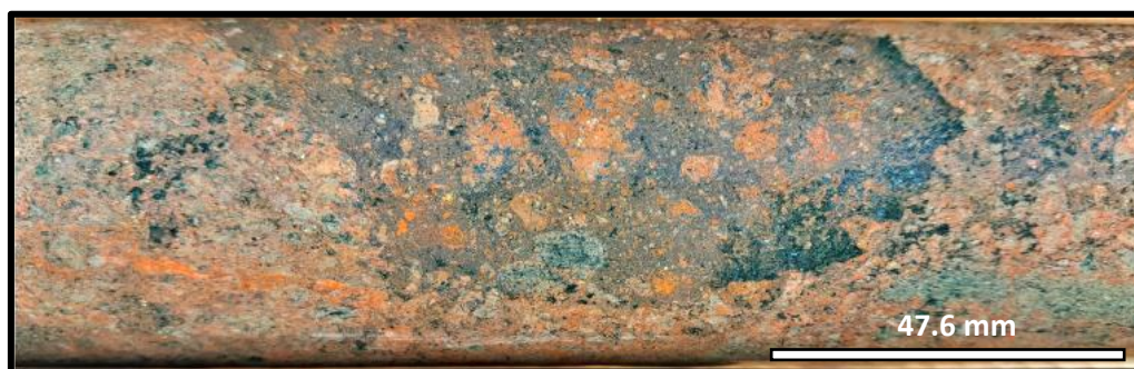
Figure 5: HWDD08 1029.2m. Granite-gneiss with weak red feldspar-sericite alteration, partially brecciated with grey haematite-strong disseminated chalcopyrite-pyrite matrix infill.
