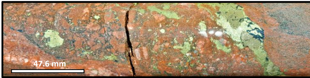
Figure 6: HWDD08 1040.7m 2cm massive chalcopyrite >pyrite-minor magnetite vein, with 5cm magnetite-chalcopyrite-pyrite breccia in footwall.
