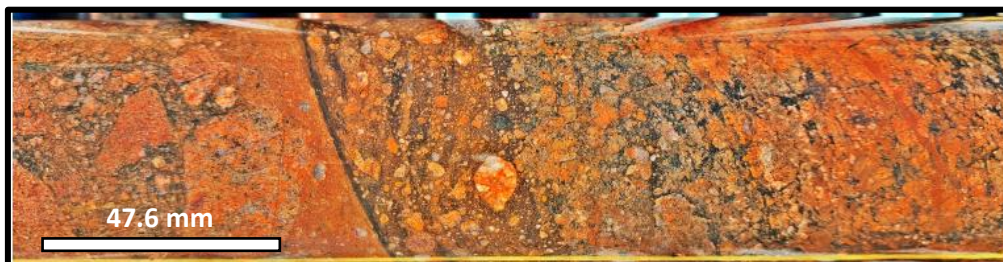
Figure 7: HWDD08 961.3m. 3cm planar milled breccia in polymict breccia zone. Sedimentary-gneiss with some granite-gneiss clasts.
