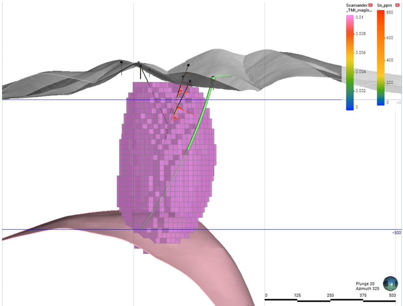
**Figure 3 - North Scamander Prospect Cross Section (looking NW) – Proposed drillhole NSD005, Historic drillholes with tin grades , modelled granite surface (pale pink) and Magnetic Inversion ( $0.015$  to  $0.59 \times 10^{-5}$  SI units) (bright pink)**
