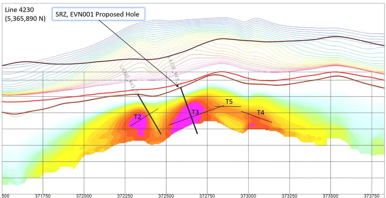
Figure 9 - Evenden Prospect Cross Section, Flight Line 4320 (5,365,890 N) - Resistivity Depth Image (RDI), Surface Topography (brown line), EM TAU dB/dt Z Profile (above topography), Modelled Plates and Proposed Drillhole (Source: EL22/2010 Yunnan Tin 2015 Annual Report, Appendix 5)
