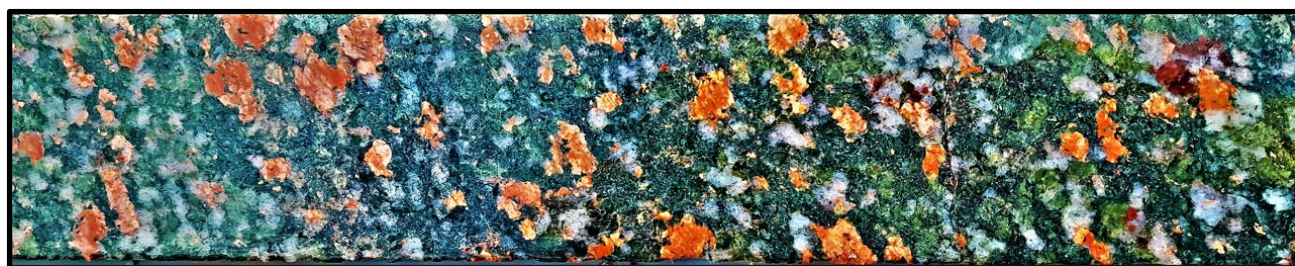
Figure 7: HWDD03 1015.8m Donington Granite with green chlorite after mafic minerals and green sericite on brown sericite after smaller feldspars. Relict coarse feldspar phenocrysts with red feldspar and eroded sericitic margins.
