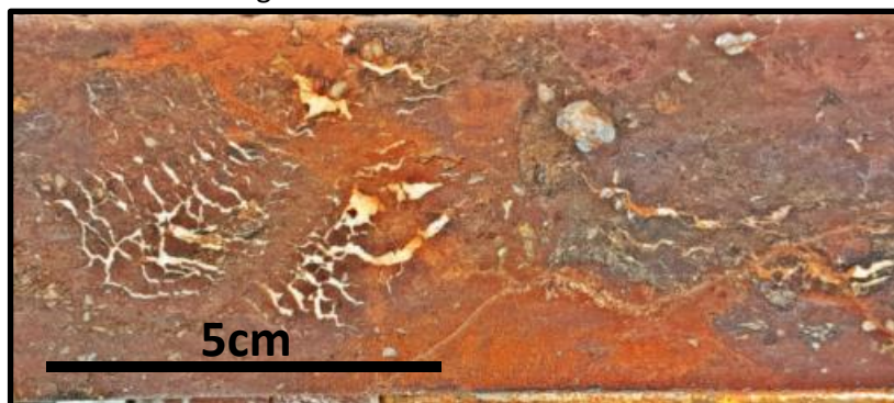
Figure 5: HWDD03 1044.4m. Pale silica with yellow sericite hue, fine crackle with red-brown haematite infill. White siderite stringers.
