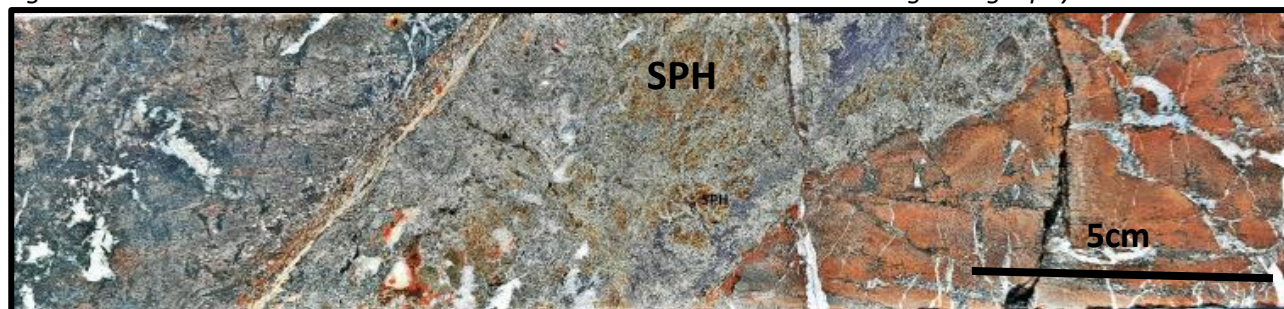
Figure 2: PSDDH01 865.55m 6cm fault with massive pale brown sphalerite-galena infill
